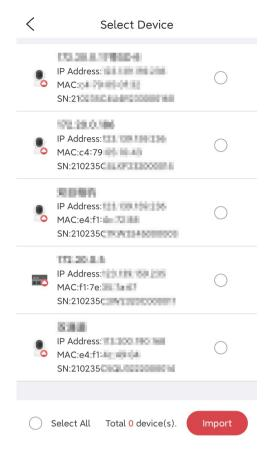
5. Tap **Import** to complete adding the device. The device will be deleted from its previous project (except when the previous project is the default project).
